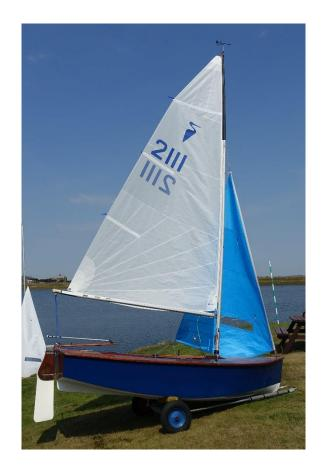
All wooden construction, built circa 1960, completely refurbished, redecked and epoxy coated late 1980's.
